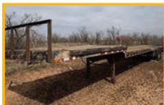
EQUIPMENT TRAILER, TOP DECK 164", BOTTOM DECK 32", DOVETAIL FOLDING RAMPS
